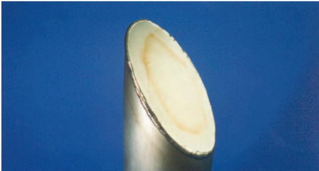
Abb. 8: WIG-Ecknaht an Ti-6Al-4V
